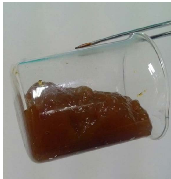
Figure 8. The status of the gel after 30 days at 200°C. [Color figure can be viewed in the online issue, which is available at wileyonlinelibrary.com .]
